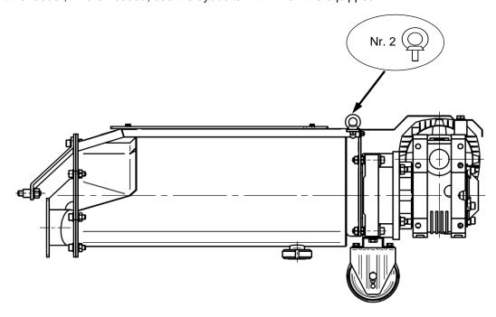
The wheels supplied are suitable for short movements of a few meters only, to facilitate connection and disconnection to the associated pump.
