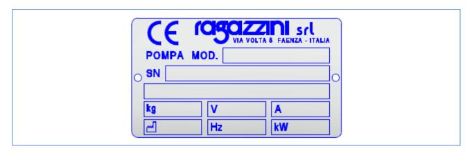
**PLEASE NOTE**: All the data marked on the plate must always be legible. Refer to the identification data in all communications with the manufacturer, e.g., requests for replacement parts, information, and technical assistance. If the plate deteriorates with use and is no longer legible, even in only one of its elements, another one must be requested from the manufacturer, by referring to the data contained in this manual or on the original plate.
