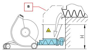
**MOVING PARTS HAZARD:** display the warning signs on the sides giving access to the feeder.
